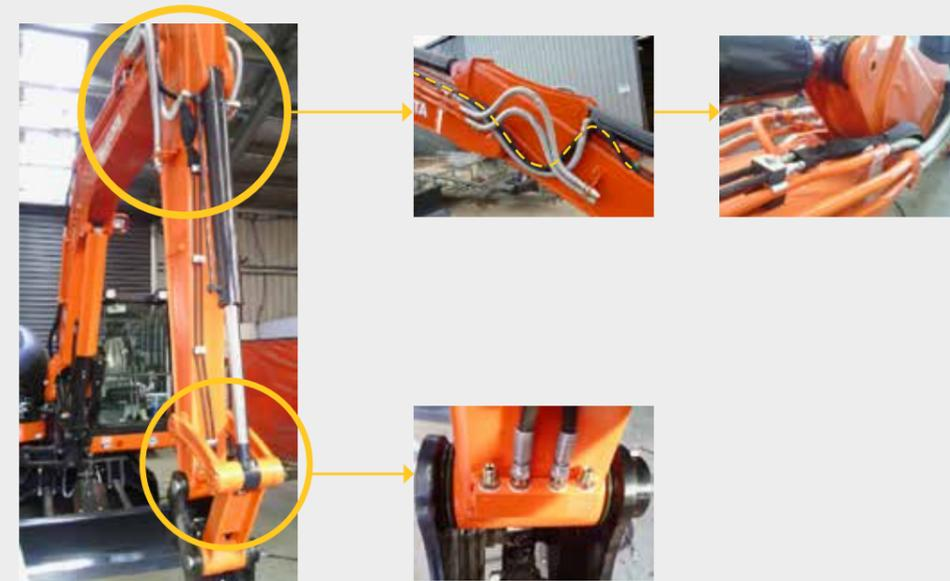
18. Run 2x mm hose up dipper arm, using mm hose clamps to secure them in place as shown in photo
