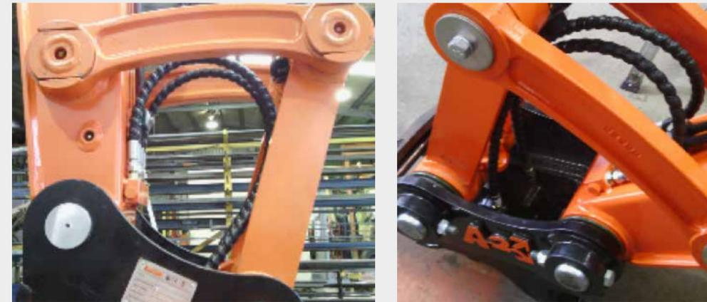
17. Run 2x mm hose up dipper arm, using mm hose clamps to secure them in place as shown in photo
