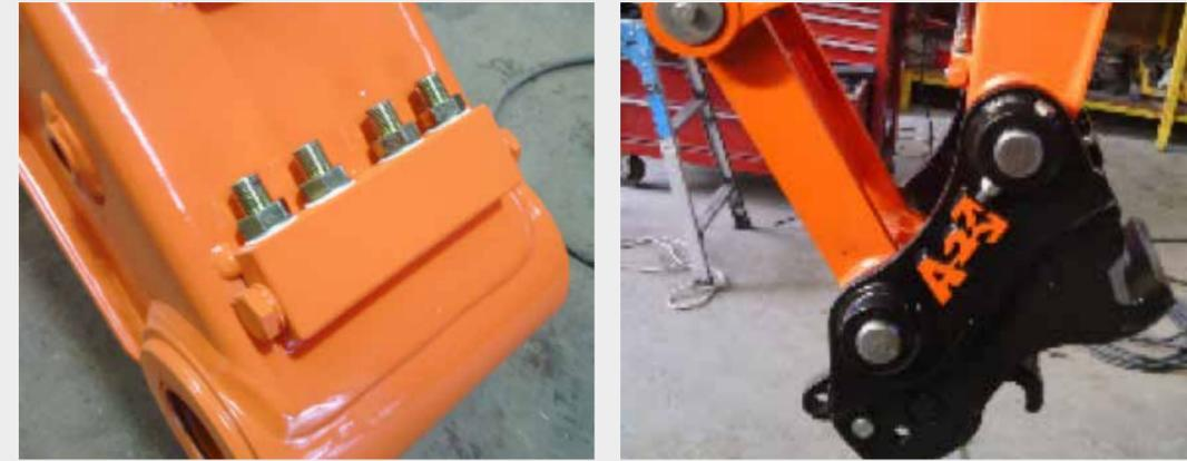
16. Run 2x short hoses with protective wrap from manifold to hitch
